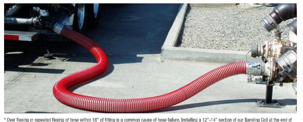
the hose should be considered. *Kanaflex will not be responsible for damage to hose due to over flexing.*
